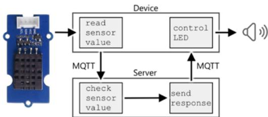
One real-world use of this setup would be in a large indoor space with many temperature and humidity sensors, such as a farm. Before deciding to turn on air conditioning, data can be gathered from multiple temperature and humidity sensors. If only one sensor reading exceeds the threshold, but other sensor readings are normal, this can prevent the entire air conditioning system from being turned on.
