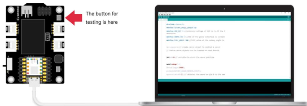
Note the position of the buttons on the XIAO extensions used for testing in the figure.
