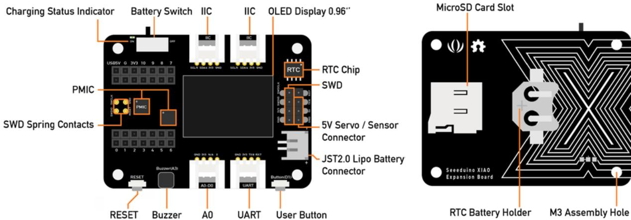
This expansion board enables the building of prototypes and projects easily and quickly, using its rich peripherals such as OLED Display, SD Card interface, RTC, passive buzzer, RESET/User button, 5V servo connector, and multiple data interfaces.
