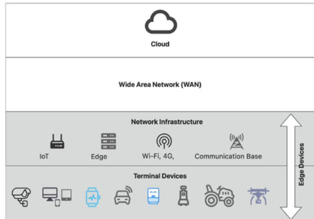
Devices at the network edge can communicate with the cloud, edge infrastructure, and each other. Edge applications typically span multiple locations on this map. For example, data may be sent from an IoT device equipped with sensors to a local edge server for processing.
