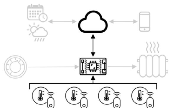
temperature sensor and may connect to multiple external temperature sensors via wireless protocols such as Low Energy Bluetooth (BLE).
