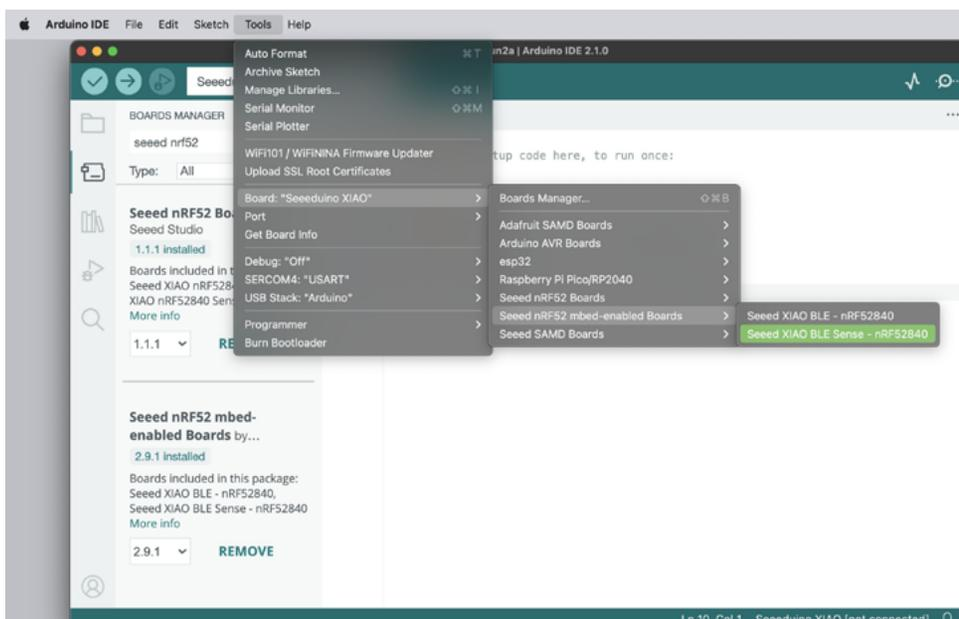
Your development board is now ready to run code on it. Let's start with Blink - lighting up the LED. Note that the board does not have a regular LED like most Arduino boards. Instead, you will find an RGB LED that can be activated with "reverse logic" (you should apply LOW to activate each of the three separate LEDs). Test your RGB LED with the following code:
