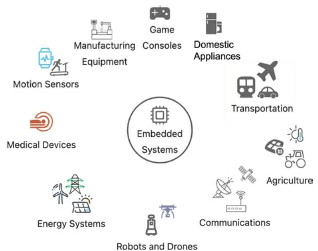
Embedded systems can be large or small, as small as the microcontroller controlling the digital watch and as large as the embedded computer in the autonomous car. Unlike general-purpose computers such as laptops or smartphones, embedded systems usually perform a specific specialized task.
