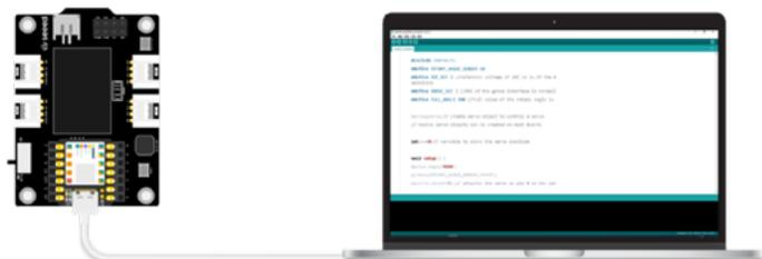
Once connected, click on the “Upload” button to upload the program to the hardware. When the debugging area displays “Upload Successful”, check if the OLED display screen has shown a circular pattern.
