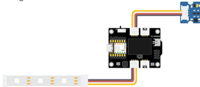
Use a data cable to connect XIAO to your computer, click the “Upload” button in Arduino IDE, and upload the program to the hardware. Once the debugging area shows “Upload Successful”, you can open the serial monitor and try swinging the three-axis accelerometer left, right, up, and down to feel the light effect changes of the light strip.
