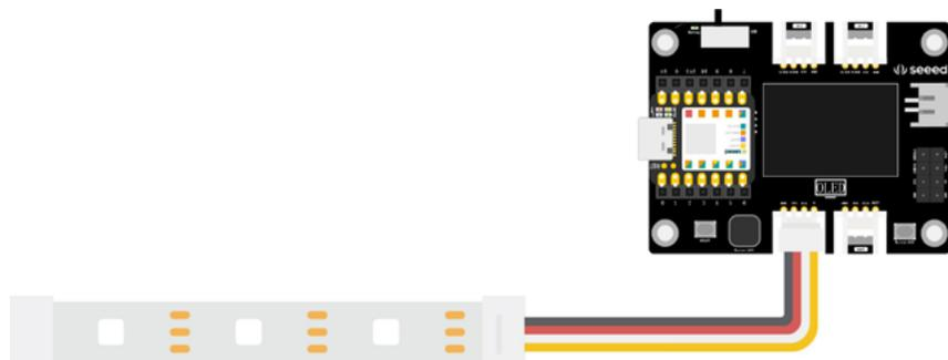
The light strip can change color, flicker, and present various lighting effects such as breathing. We can refer to the sample program in the library: **File** → **Example** → **Adafruit NeoPixel** → **buttoncycler**. This sample program switches different lighting effects on the light strip through buttons. We can find the code for various lighting effects in it, such as flickering, rainbow lights, chasing, etc.
