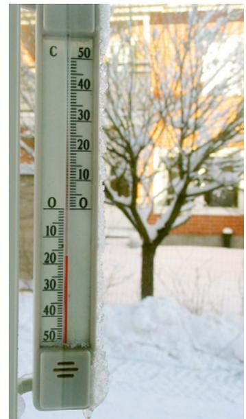
Furthermore, the phenomenon of thermal expansion and contraction is often used in temperature measurement. Commonly seen thermometers and body thermometers are based on the principle of measuring temperature by the expansion and contraction of a liquid when heated or cooled. The image below shows a commonly used alcohol thermometer that measures temperature by the property of alcohol's expansion and contraction with temperature. The winter daytime temperature displayed in the image is -17°C.
