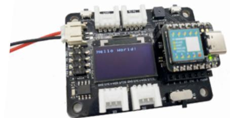
Click "Upload" to transfer the program to the main control board. Once the upload is complete, check if the OLED display shows "Hello World!".
