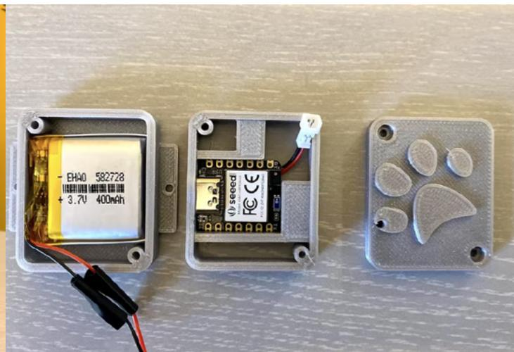
This project is a wearable device that tracks pet activities using XIAO BLE Sense and Edge Impulse, aimed at helping our pets stay active. The XIAO BLE Sense is a mini controller equipped with a powerful Nordic nRF52840 MCU, built-in Bluetooth 5.0 module, and designed around a 32-bit ARM® Cortex™-M4 CPU. It features a 6-axis IMU that can be used to predict activities such as rest, walking, and running.
