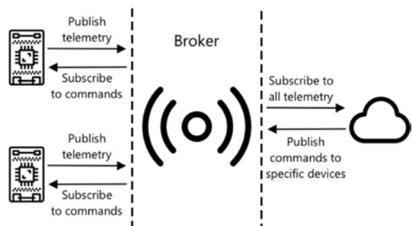
MQTT is the most popular communication protocol for IoT devices and will be covered in this section. Other protocols include AMQP and HTTP/HTTPS, which we introduced in the previous section.
