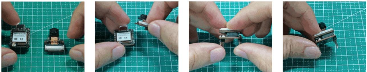
As commented in the introduction, the expansion board, or the “sense” part of the device, has a 1600x1200 OV2640 camera, an SD card slot, and a digital microphone.
