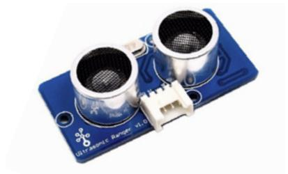
The ultrasonic receiver stops timing as soon as it receives the reflected waves. The actual distance from the emission point to the obstacle is calculated based on the time difference between emission and reception, much like bat echolocation. The application range of ultrasonic waves is becoming broader, commonly seen in reverse radar systems, intelligent guidance systems, robot obstacle avoidance systems, medical ultrasound examinations, and more.
