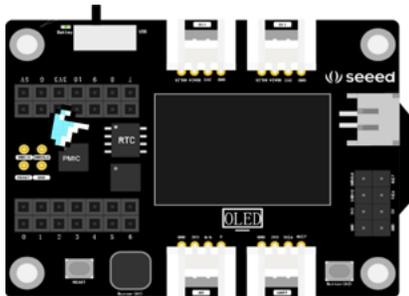
Position of the RTC clock chip on the XIAO expansion board
