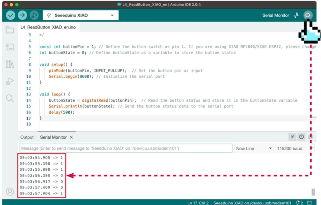
When we press the button on the XIAO expansion board, the serial monitor shows **0**, and when we release the button, the serial monitor shows **1**.
