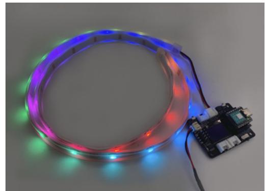
Use a data cable to connect XIAO to the computer, click the “Upload” button, and upload the program to the hardware. When the debugging area shows “Upload successful”, you can observe the light effect of the light strip.
