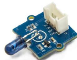
Grove - Infrared Emitter Infrared Transmitter Module
