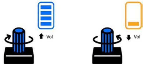
The rotary potentiometer can produce an analog output value between 0 and VCC (the voltage of the connected circuit) on its connected pins. By rotating the knob, you can change the output voltage value. The range of the knob's angle is 300°, and the output value is 0-1023. We can use the rotary potentiometer to control the LED light to show brightness changes, or control the servo to rotate at different angles, etc.
