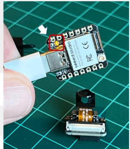
*Note that the pins work with inverted logic: LOW to Turn on and HIGH to turn off.*
